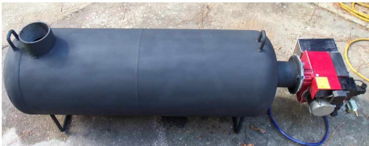
Burner installed on a furnace fabricated from a scrap propane tank.
