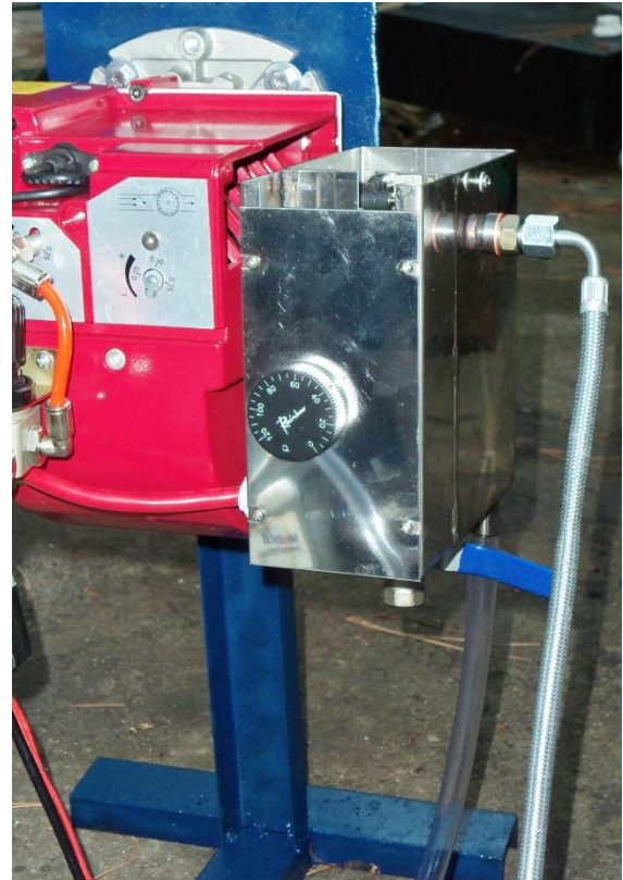
Oil Reservoir Tank with Input line
