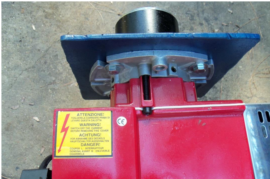
Burner Flange Installed on Burner
